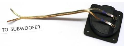
Strip ends of included wire. Attach crimp terminals to one end and connect to terminal cup as shown.
