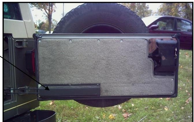
This particular photo represents '76-'02 models and this close-up has three black squares representing the approximate positions that the knob pieces for the hangers will install and where the rubber bumper rests:
