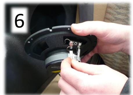
With the tape used as a marker still on the carpet, make a small slit about an inch past the tape so the wire will poke through **under** the pod when it's installed. Run your speaker wire from your radio or amplifier under the carpet and up through slit so about a foot or wire exits. The wire should only be **under** the pod in that tiny area and should be away from the pod after that so you get the best fit. Repeat process for the other pod.
