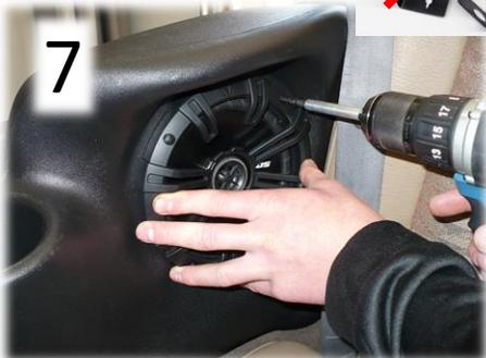
**#120998 & #120998-K65:** Center speaker in hole and get any logos in desired position. Hold speaker firmly in desired position and use drill with Phillips bit to screw speaker in place. Repeat process for other pod.
