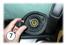
Push excess wire through pod and down into dash. Line up speaker to the screw holes and use either the screws that came with your speakers or the stubby black screws we provide if you prefer (recommended).
