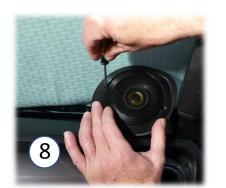
Line up grille holes to the pre-drilled holes in the pod and screw grille in place. Do the two lower screws first. A pick-awl can help to locate the holes.
