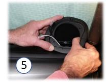
Pull connector wires up through pod. Drop pod onto the clips from #3, then push pod down over ribs of retaining clips until pod is fully seated. A flashlight can help in lining up the holes. You can gently bend one or more clips in the direction needed if necessary.
